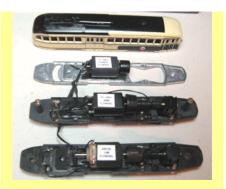
he first chassis, shown directly under the Body shell, uses that is the current Bowser motor with the A-line 20040 Although not readily apparent here, a new drive shaft and drive line parts based on Stewart designs is also part of the package. The latter combination is under test and evaluation by Custom Traxx and the Southern California Traction Club and looks like a winner.
